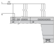
(1) 1 A quick-blow fuse or circuit-breaker. NOTE: QF and QG: 5 A for SR3XT141--
